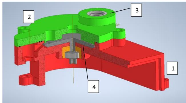
**Fig. 2.** The design of feeding system: 1 – base, 2 – base cover, 3 – threaded sleeve, 4 – disc.
