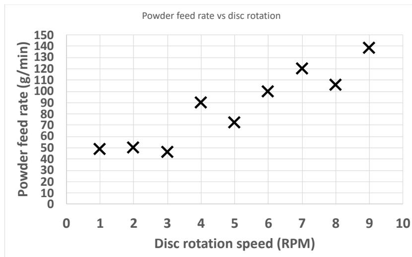
**Fig. 8.** The relationship between disc rotation speed and powder feed rate.
