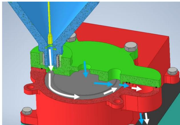
**Fig. 3.** Motion diagram of carrier gas (blue) and powder (white).
