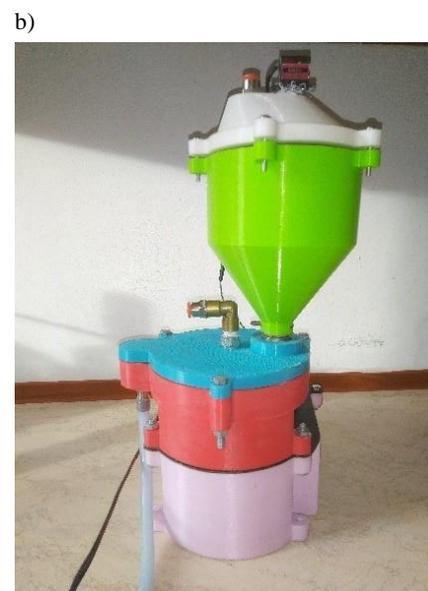
**Fig. 6.** a) front and b) back view of powder feeder after assembly.
