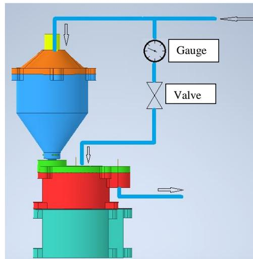
**Fig. 5.** The scheme of carrier gas flow.
