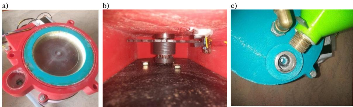
**Fig. 7.** Individual components after assembly: a) interior with drive, b) threaded bushings, c) drive system with speed sensor.
