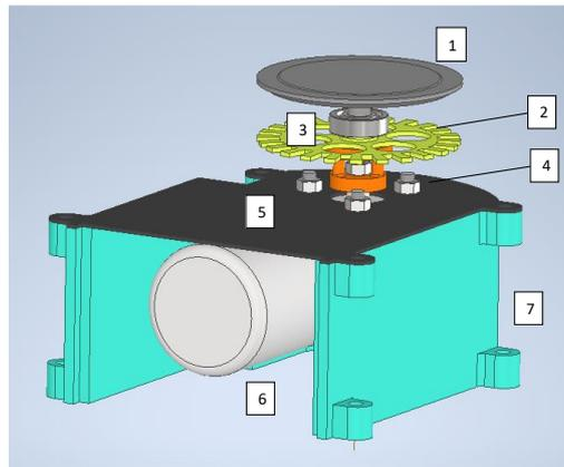
**Fig. 4.** Scheme of powder feeder drive system: 1 – disk, 2 – bearing, 3– serrated wheel, 4 – claw coupling (active and reactive parts), 5 – disc, 6 – motor with worm gear, 7 – motor cover.
