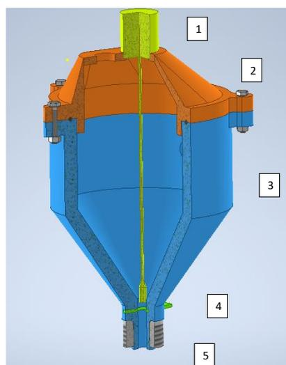
**Fig. 1.** The scheme of powder hopper: 1 – motor 5 V with agitator, 2 – container cover, 3 – container, 4 – cap, 5 – sleeve with male threads.
