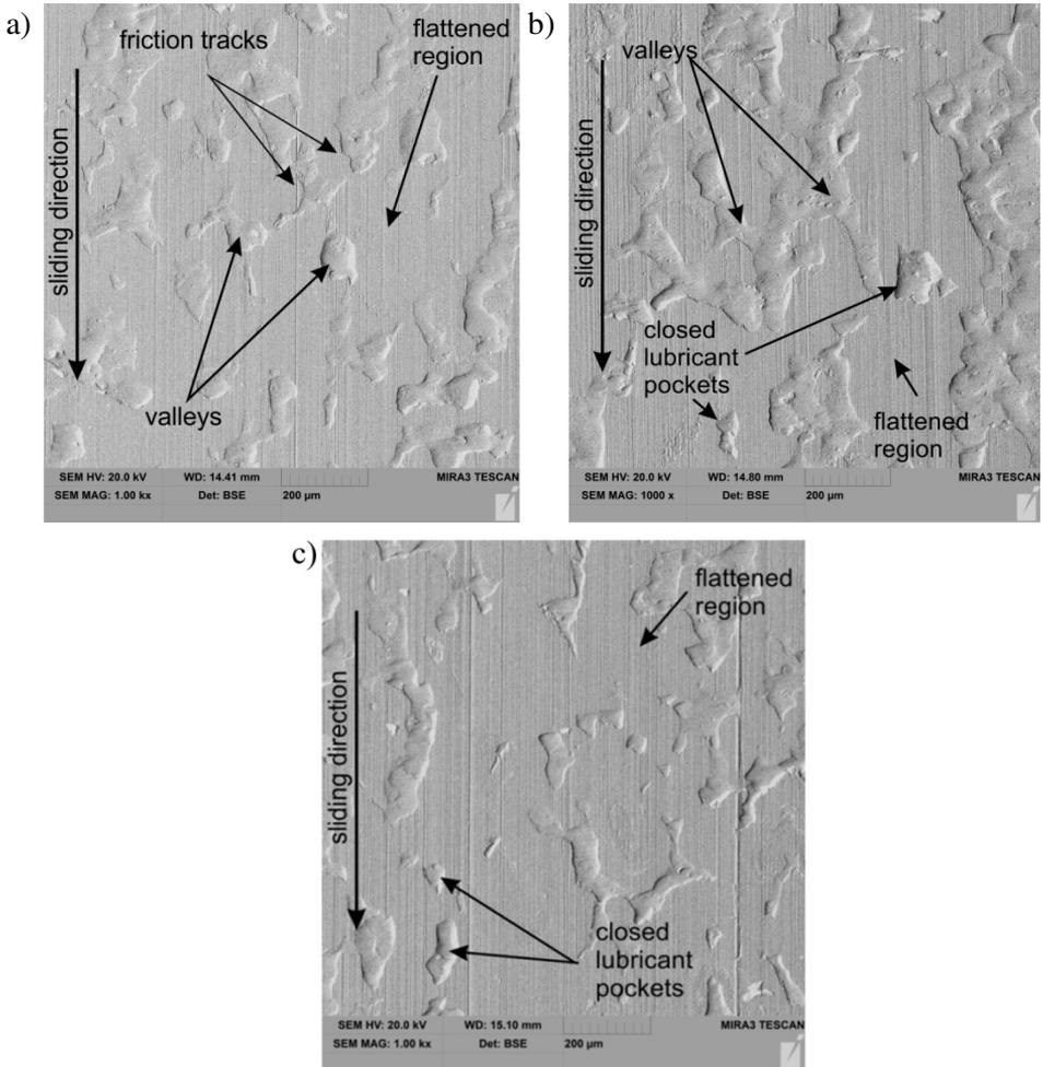
Fig. 5. SEM micrographs of sheet metal surfaces tested under a load of 9 [MPa] in conditions of: a) dry friction, b) lubrication with machine oil and c) lubrication with gear oil
