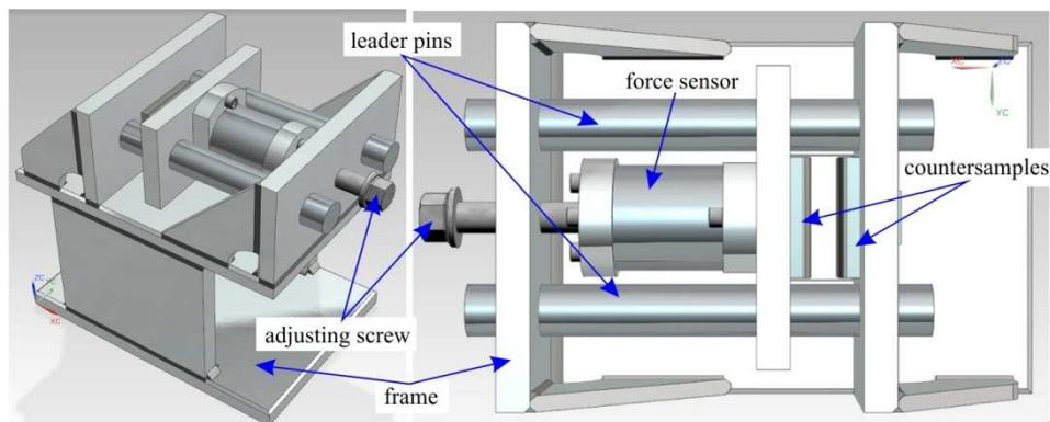
Fig. 2. Model of the friction tester
