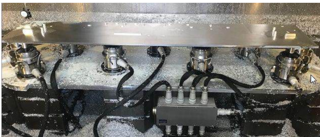
Fig. 6. Developed method of mounting an element on a CNC machine in OP20.
