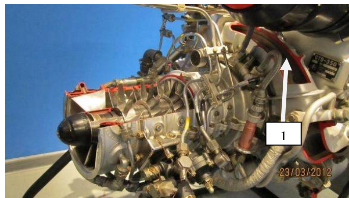
Fig. 1. Axial-centrifugal compressor of turboshaft engine GTD-350 - a gift from WSK PZL Rzeszów to the Rzeszów University of Technology: 1 – double jet collector.
