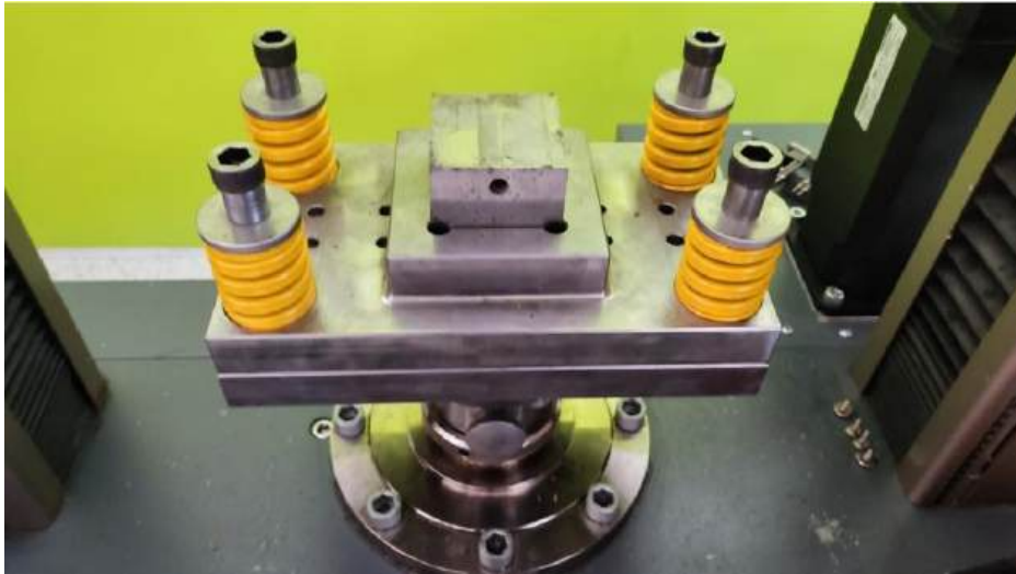
Fig. 4. The U-draw bending tool mounted on a testing machine.
