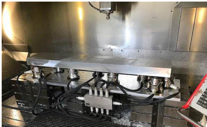
Fig. 3. Developed method of mounting the blank on a CNC machine in OP10.
