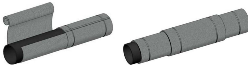
Fig. 5. Pipeline insulation using aerogel
