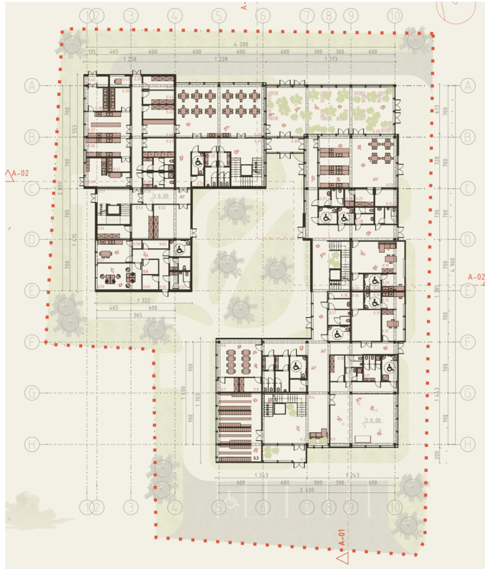
Fig. 9. Ground floor plan of a kindergarten that combines integration functions with senior citizens in Grodzisko Dolne. Source: elaborated by Zuzanna Chmura
