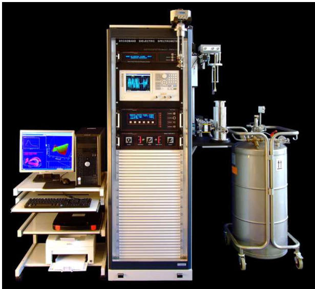
Fig. 9. Dielectric spectrometer Novocontrol ALFA-A used in dielectric measurements
