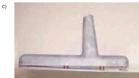
Fig. 8. Images of the trowel handle destruction during the bending and torsion trial with the load parallel to the working area of the trowel: a) and b) aluminum alloy handle, c) polyamide handle, d) polystyrene handle
