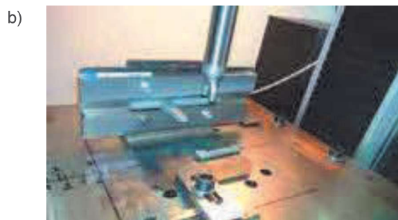
Fig. 7. Bending and torsion trial with a load parallel to the working surface of the trowel (polyamide handle): a) the mounting of the trowel and the load application, b) termination of the trial – handle breaking
