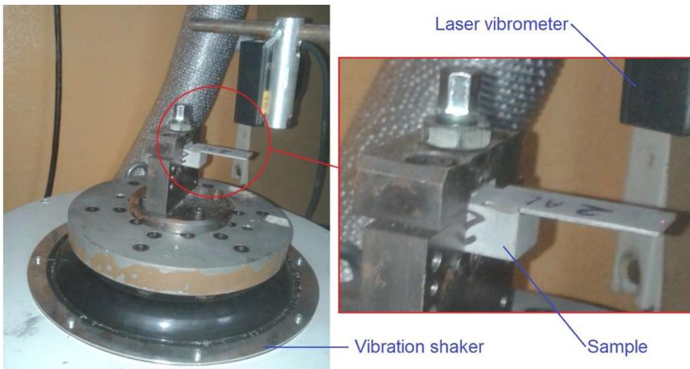
Figure 4. Setup for fatigue testing of adhesive joints
