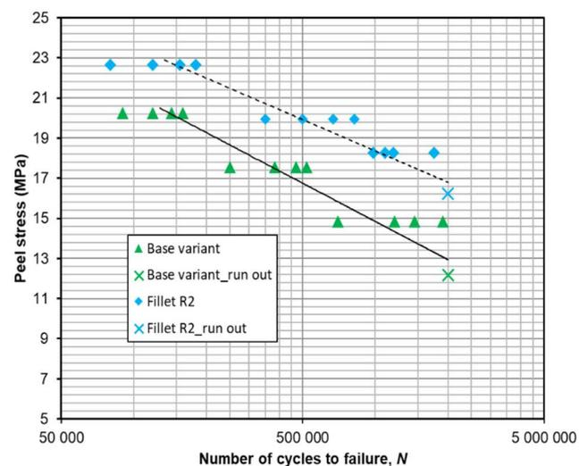
Figure 5. Comparison of the fatigue curves for the base variant and fillet R2 variant
