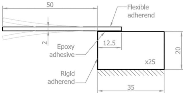
Figure 1. Shape and dimensions (in mm) of adhesive joint samples used in fatigue tests
