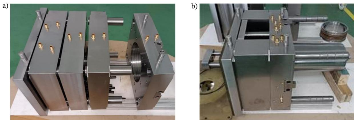
**Fig. 7.** Modular injection mould with a conformal cooling channel for the production of hydraulic filter housings: a) die (during assembly); b) punch
