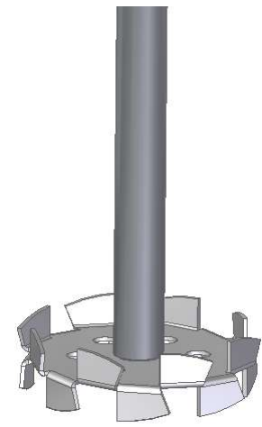
Fig. 4. Dispersing disc agitator used in the tests
