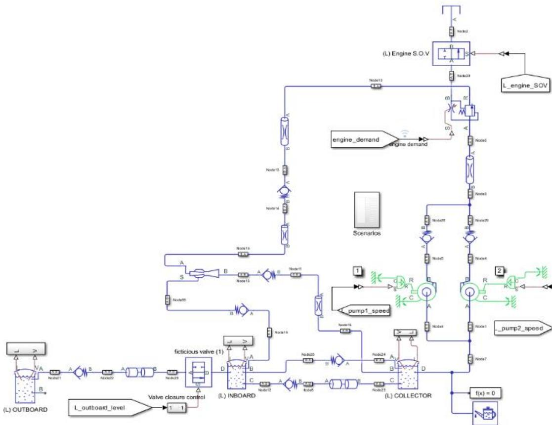
Fig. 2. Fuel system model in Simulink Simscape environment
