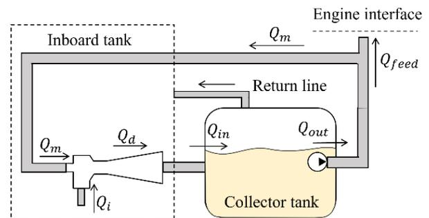
Fig. 6. Jet pump and collector tank flow balance
