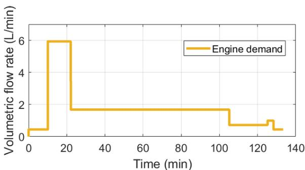
Fig. 11. Engine demand for a simplified typical flight envelope
