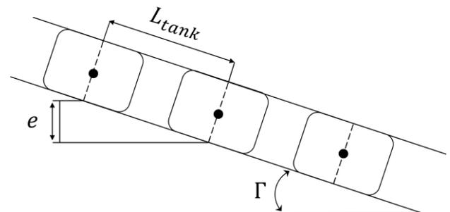
Fig. 4. Pipe elevation proposed model
