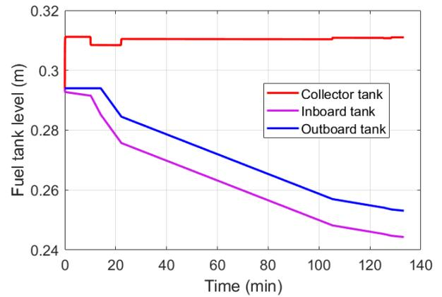
Fig. 12. Fuel tank levels for zero dihedral configuration
