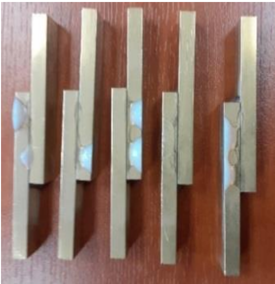
Fig. 16. A batch of brass samples bonded with Epidian 57 / Z1 adhesive
