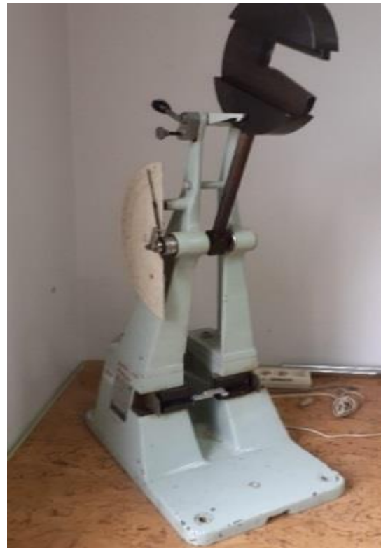
Fig. 15. Sample placed on a pendulum hammer
