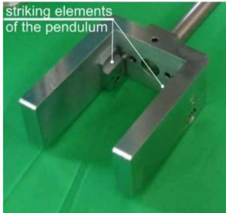
Fig. 6. Modified striker of a hammer
