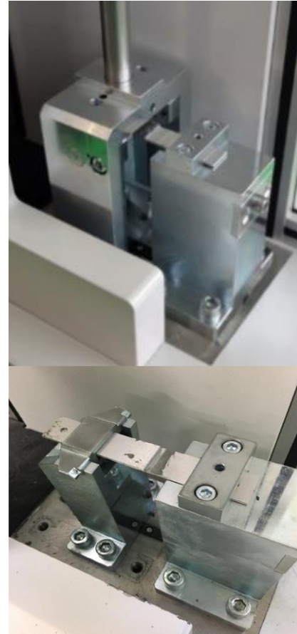
Fig. 8. The sample attached to the impact tests
