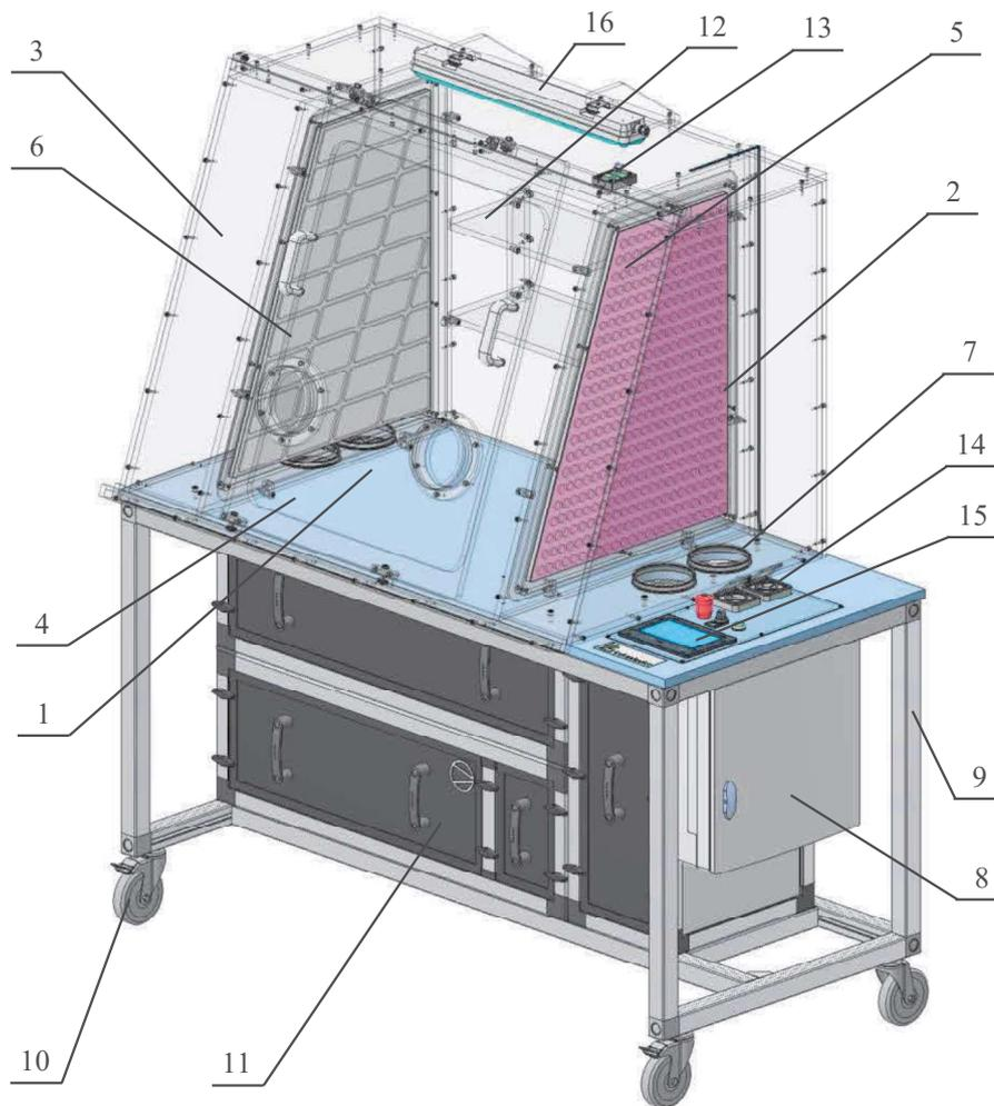
**Fig. 2.** 3D virtual model of the laminar flow cabinet (front view): 1 - workspace, 2 - inlet chamber, 3 - outlet chamber, 4 - sliding doors, 5 - inlet partition (right), 6 - outlet partition (left), 7 - inlet channels, 8 - control system cabinet, 9 - frame, 10 - caster wheel with lock, 11 - ventilation module, 12 - shelves, 13 - cable gland, 14 - power sockets, 15 - control panel, 16 - LED lighting
