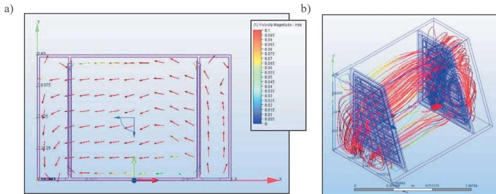
**Fig. 4.** The result of the airflow simulation in the cabinet: a) velocity distribution in the inlet, workspace, and outlet chambers, b) airflow distribution (view from the outlet chamber side)
