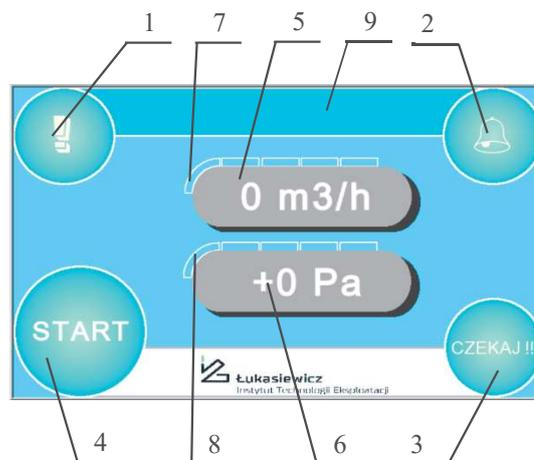
Fig. 7. View of the control panel: 1 - warning icon, 2 - alarm icon, 3 - ready-to-operate icon, 4 - device activation icon, 5 - information about current airflow rate, 6 - information about current pressure difference between the cabinet and the surroundings, 7 - barograph of the percentage efficiency of the supply fan, 8 - barograph of the percentage efficiency of the exhaust fan, 9 - field with information about alarms, warnings, and current events
