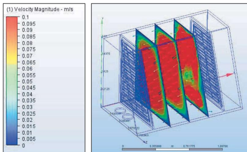
**Fig. 5.** Result of airflow simulation in the cabinet – velocity distribution in the workspace in selected vertical planes
