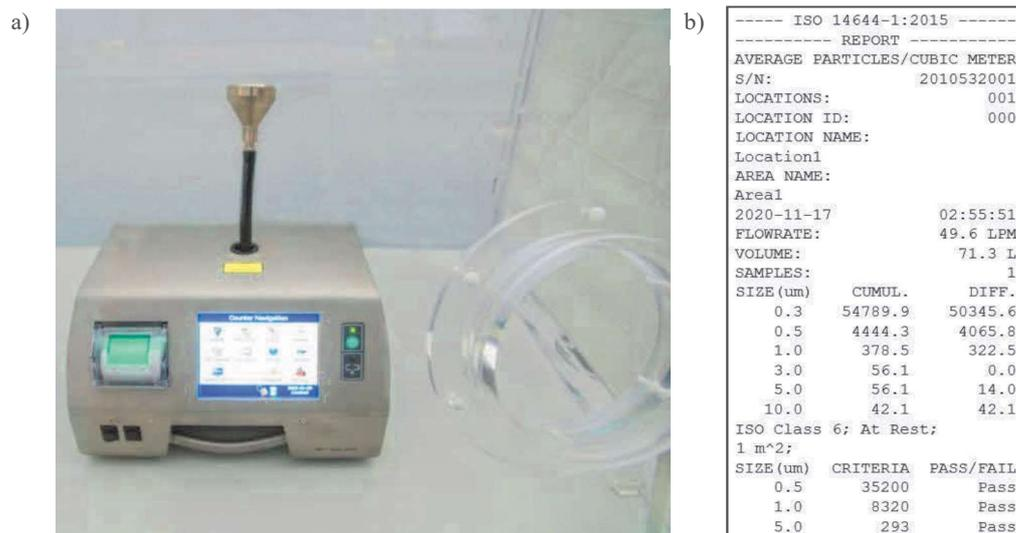
**Fig. 9.** Air cleanliness test in the working chamber using the particle counter Met One 3423 (a), and the test report for a total airflow rate of 300 m<sup>3</sup>/h (b)
