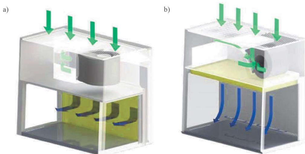
Fig. 1. Diagrams showing a) horizontal and b) vertical airflow in a laminar flow cabinet (Guide, 2024)
