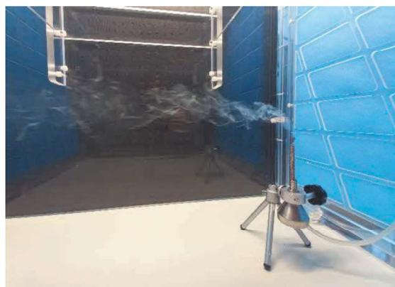
**Fig. 8.** Airflow smoke test
