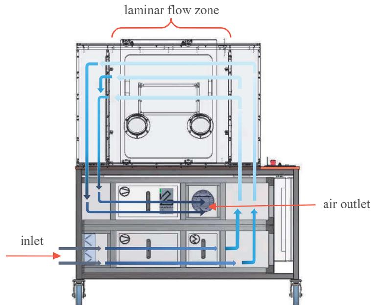
Fig. 3. Air circulation in the laminar flow cabinet
