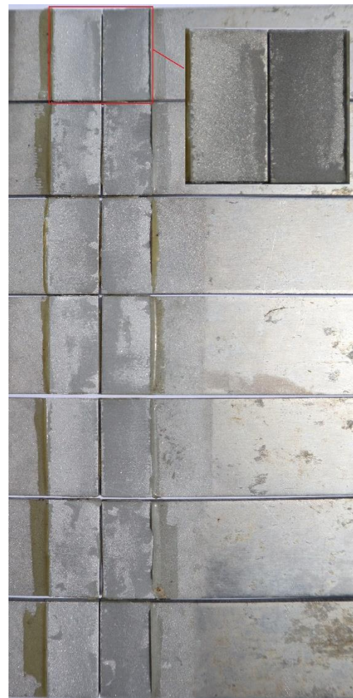
Fig. 5. Adhesive joints not subjected to shot peening and aged for 6 months from July to January
