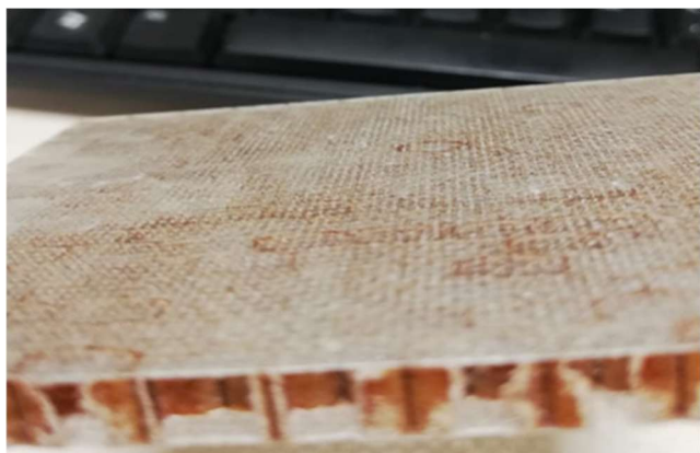
Fig. 12. View of sample loaded with 0.5 J
