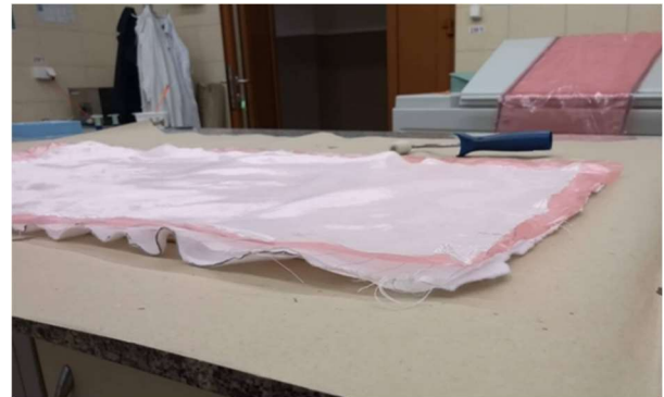
Fig. 4. Preparation process for phase II of the composite
