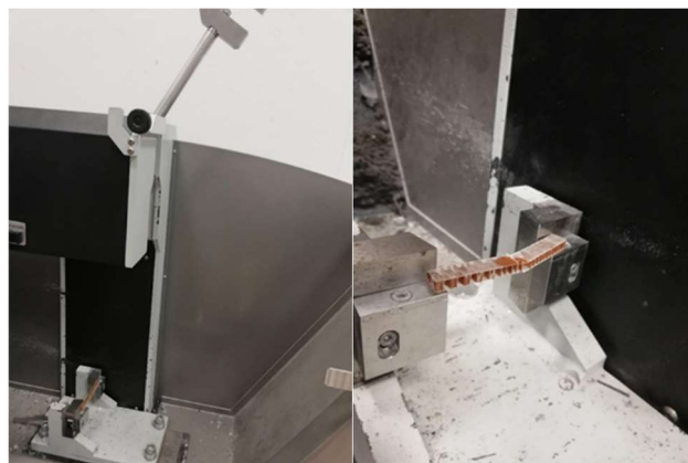
Fig. 18. Impact test under: a) plane loading, b) edge loading
