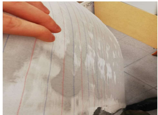
Fig. 39. Resin mostly absorbed by delamination
