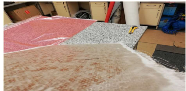
Fig. 5. Cover peeling off from the semi-product manufactured in phase I
