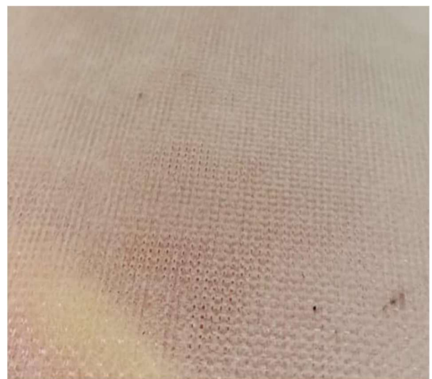
Fig. 36. Holes visible in the composite cover
