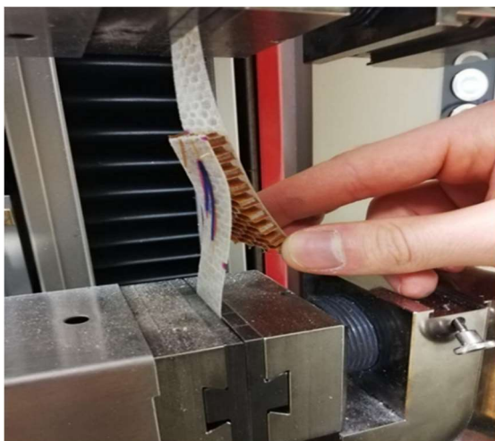
Fig. 31. Adhesion test between cover and core – Zwick/Roell 5 kN machine
