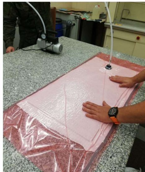
Fig. 1. Curing the composite in phase I
