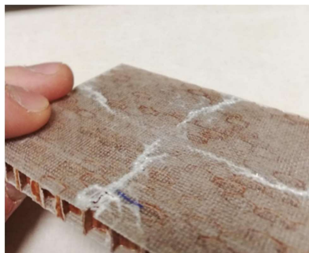
Fig. 15. View of sample loaded surface with 3 J
