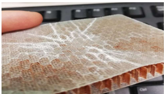
Fig. 27. Damage to a single-phase sample loaded with 5 J
