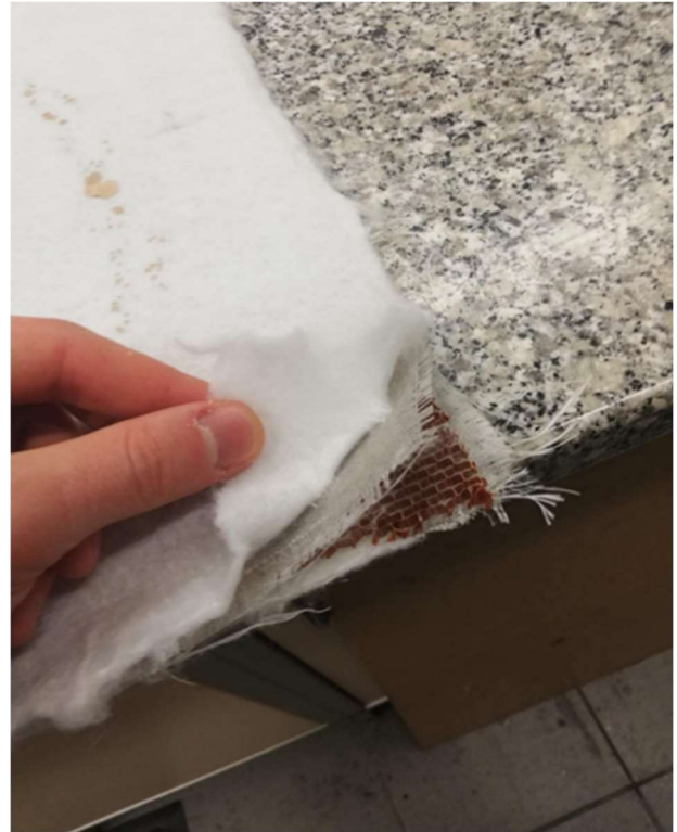
Fig. 35. Bonding of drainage mat and composite cover
