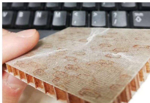
Fig. 14. View of sample loaded surface with 2 J
