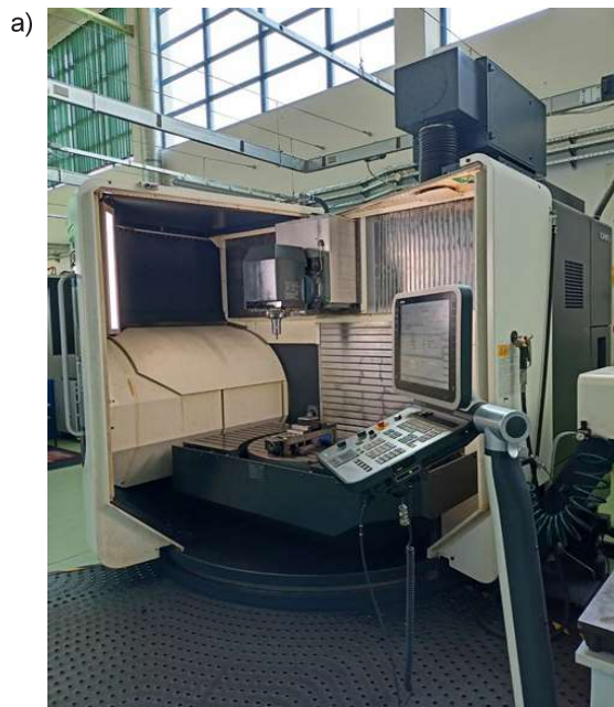
Fig. 4. Research—measurement stand: a) DMU 100 monoBLOCK milling centre. b) 3Dsystem InfiniteFocus Alicona optical microscope
