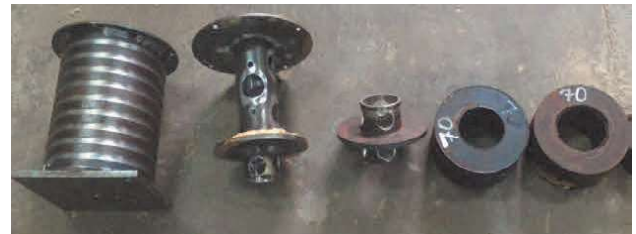
Fig. 16. Crash box elements – modification #2
