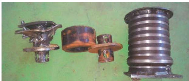
Fig. 18. Modified crash box elements deformation after the impact test
