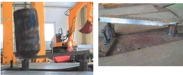
Fig. 12. Bumper with crash-boxes frame-by-frame shots – 25% side movement test.
