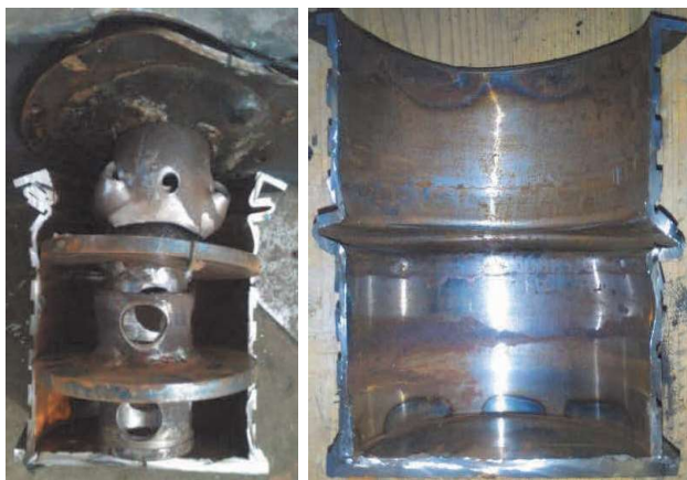
Fig. 19. Modified crash box elements deformation after the impact test (next)
