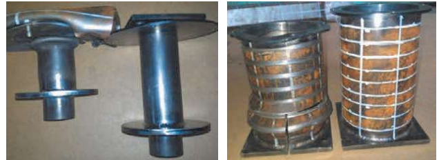
Fig. 15. Crash box elements – before and after the impact test. Modification #1
