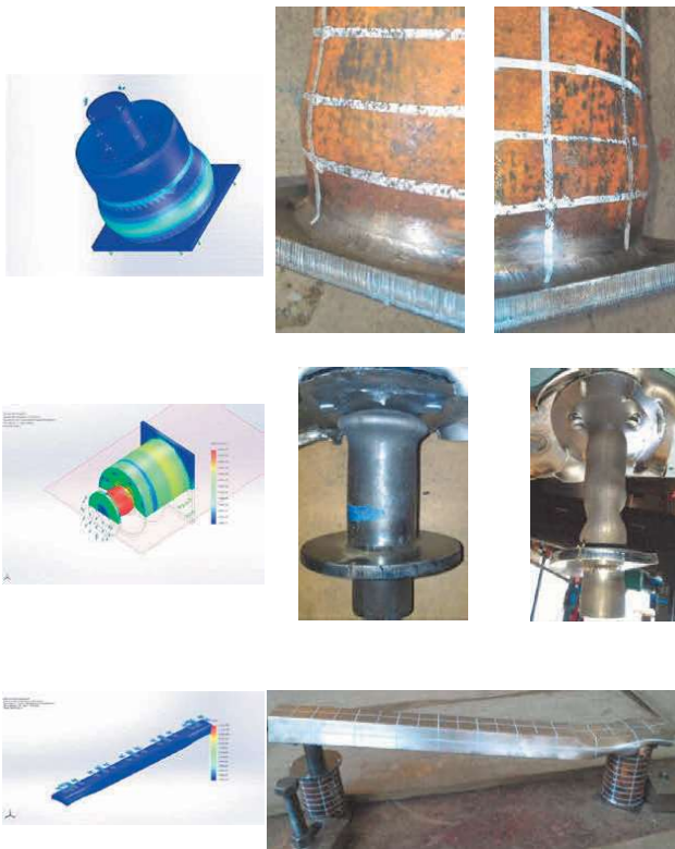
Fig. 13. Passive safety assembly with crash box–FEM simulation and site test results comparison
