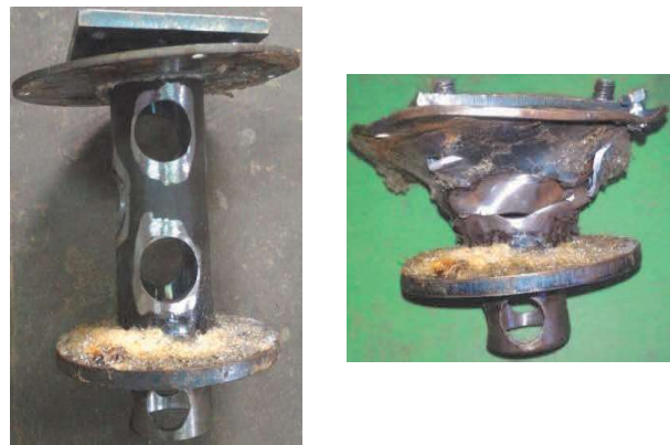
Fig. 20. Comparison of the modified crash box elements before and after the impact test
