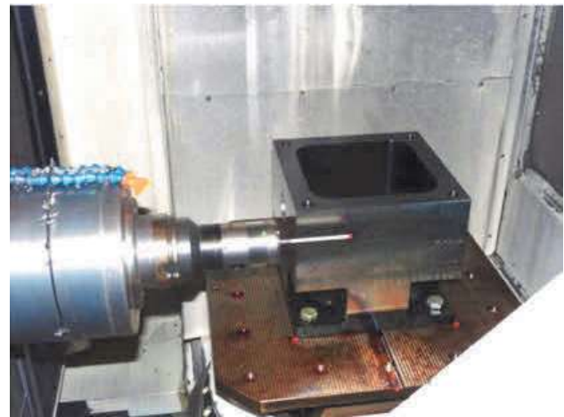
Fig. 5. View of the rectangular master part with the RMP60 object probe placed in a 4-axis horizontal machining center
