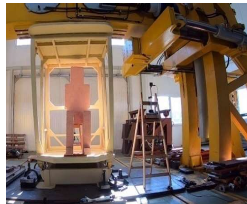
Fig. 20. ROPS structure under the vertical load
