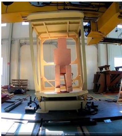
Fig. 19. ROPS structure under the lateral load
