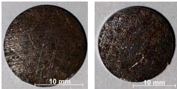
Fig. 26. Non-plastically deformed sample pieces, 17.8 mm in diameter, made up of Raex 400 steel
