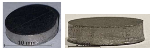
Fig. 23. Plastic deformation of a sample element, 12.6 mm in diameter, made of S235JR steel
