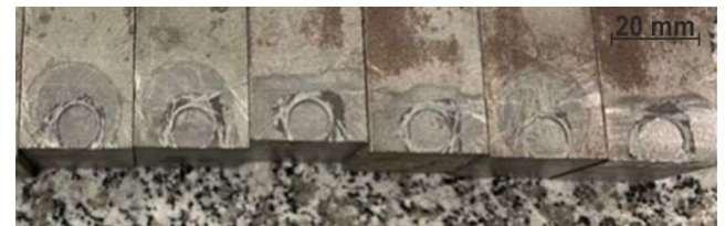
Fig. 13. Adhesive destruction of samples made up of Raex 400 material, 8.9 mm in diameter
