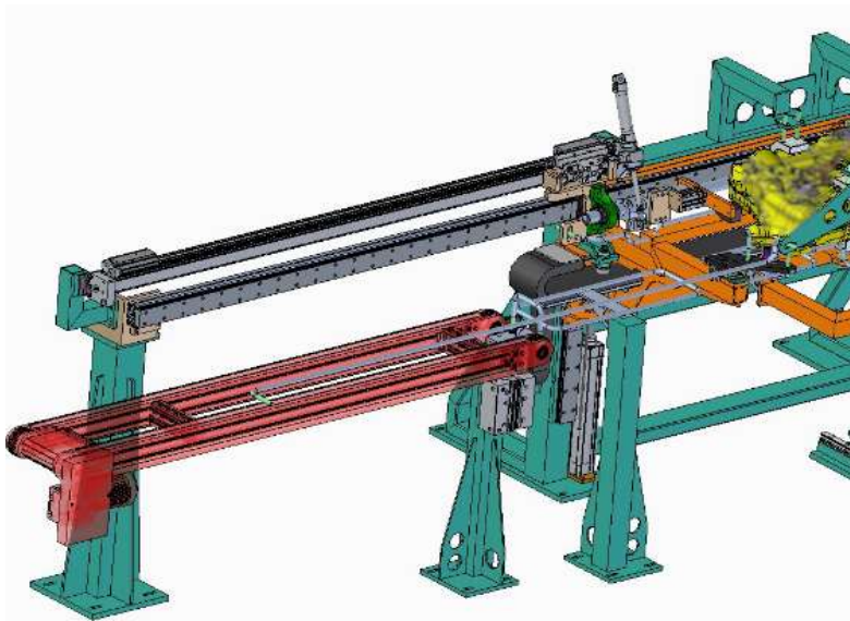
Fig. 8. Position of the feeder during tank loading
