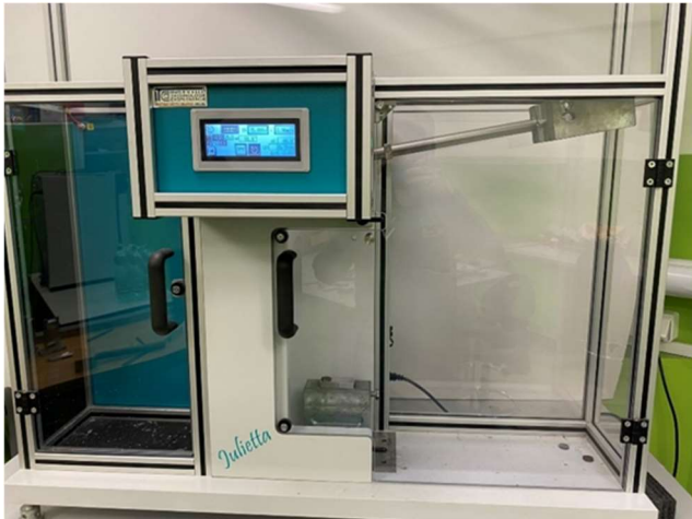
Fig. 4. "Julietta" device for testing impact strength of adhesive joints
