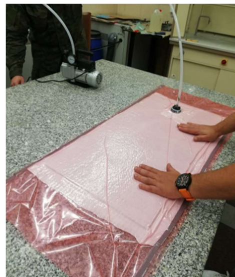
Fig. 1. Curing the composite in phase I
