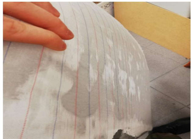
Fig. 39. Resin mostly absorbed by delamination
