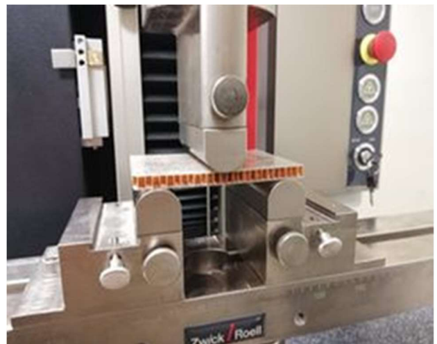
Fig. 9. Sample during a bending test – Zwick/Roell 5kN machine
