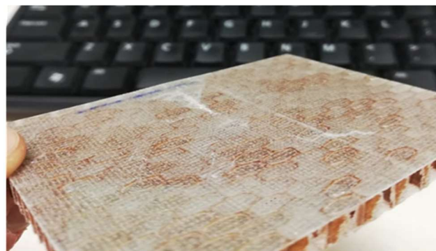
Fig. 13. View of sample loaded surface with 1 J
