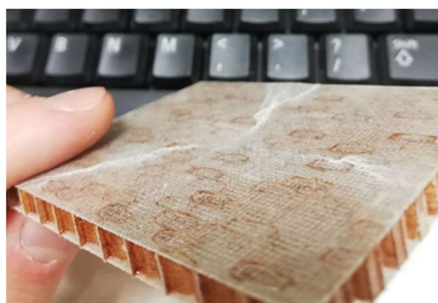
Fig. 14. View of sample loaded surface with 2 J
