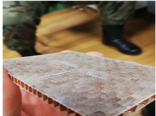
Fig. 23. View of a single-phase sample loaded with 0.5 J
