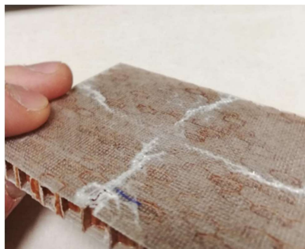
Fig. 15. View of sample loaded surface with 3 J
