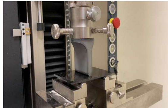
Fig. 10. Bending flexural strength test
