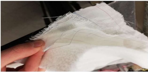
Fig. 37. Layers used in phase III of the composite
