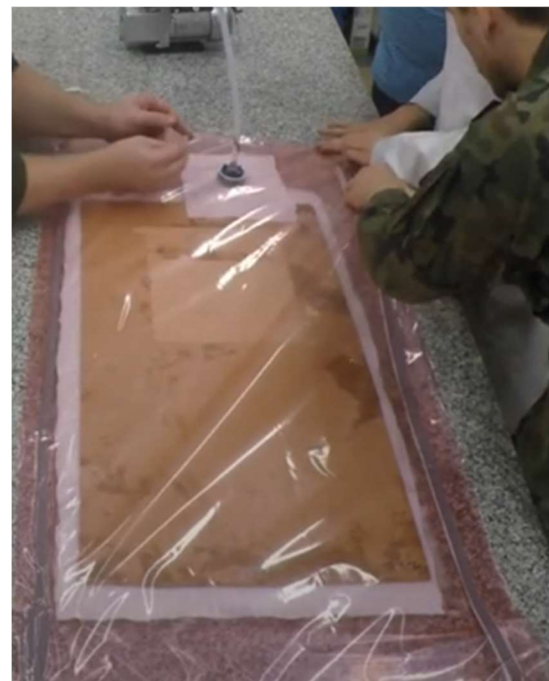
Fig. 21. Sealing off the vacuum bag
