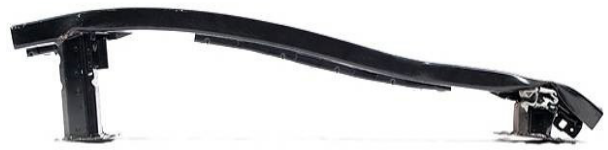
Fig. 14. Car beam with crashboxes – automotive manufacturing example
