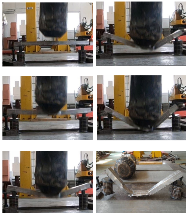
Fig. 11. Bumper with crash-boxes frame-by-frame shots – center point test.
