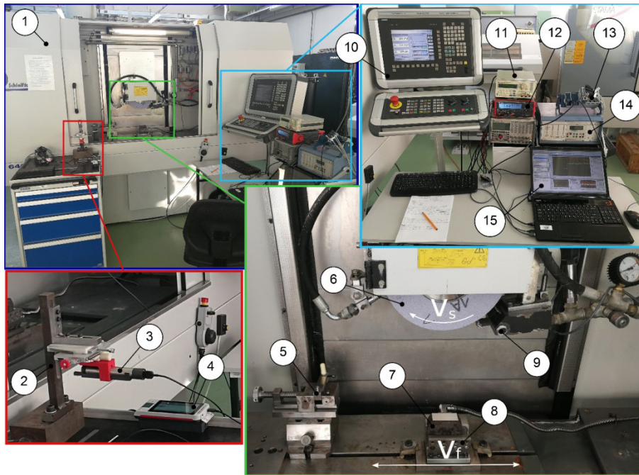
Fig. 1. Configuration of the test stand: 1 – G+H FS 640 Z surface grinding machine, 2 – mounting holder for profilometer drive unit, 3 - MarSurf PS 10 profilometer drive unit, 4 - main unit of MarSurf PS 10 profilometer, 5 – diamond dresser, 6 – grinding wheel, 7 – workpiece, 8 – dynamometer, 9 – needle nozzle for coolant distribution, 10 – machine control panel, 11 – DC power supply, 12 – desktop multimeter for coolant pressure readout, 13 – NI CompactDAQ system, 14 – Kistler 5019 A amplifier, 15 – computer with LabVIEW SignalExpress software
