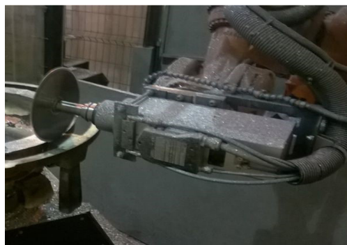
Fig. 5. Cutting off of the gating system by a robot
