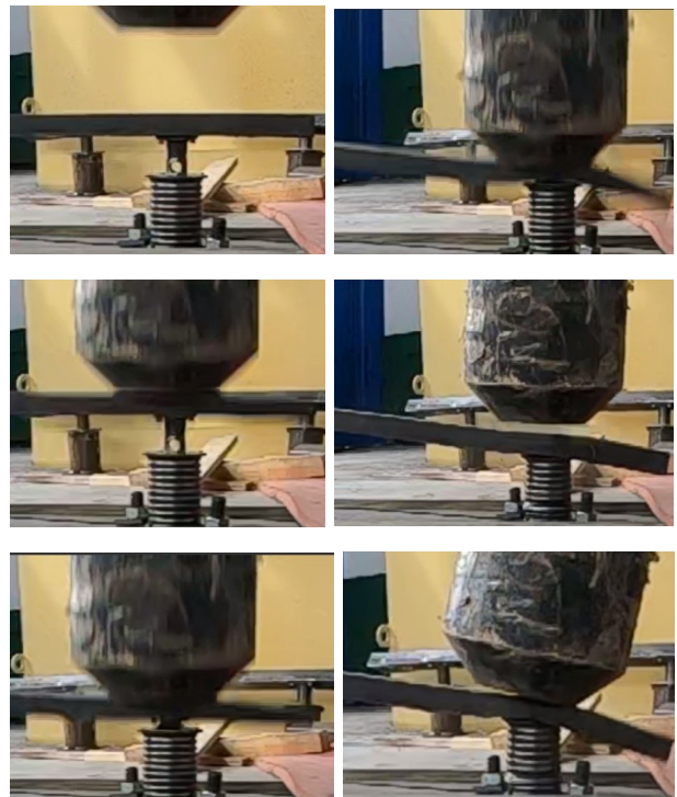
Fig. 17. Bumper with modified crash boxes – frame-by-frame impact test shots.
