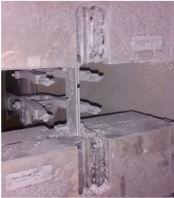
Fig. 5. Specimen view in a temperature chamber at -60°C
