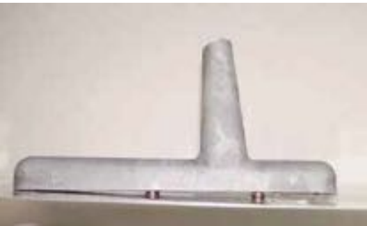
Fig. 8. Images of the trowel handle destruction during the bending and torsion trial with the load parallel to the working area of the trowel: a) and b) aluminum alloy handle, c) polyamide handle, d) polystyrene handle
