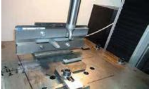
Fig. 7. Bending and torsion trial with a load parallel to the working surface of the trowel (polyamide handle): a) the mounting of the trowel and the load application, b) termination of the trial – handle breaking
