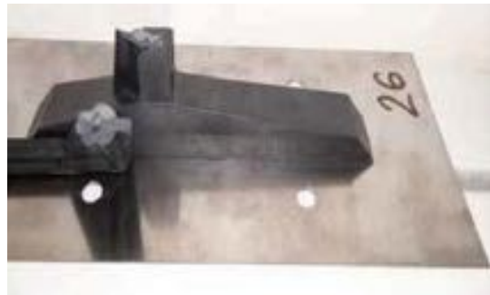
Fig. 8. Images of the trowel handle destruction during the bending and torsion trial with the load parallel to the working area of the trowel: a) and b) aluminum alloy handle, c) polyamide handle, d) polystyrene handle
